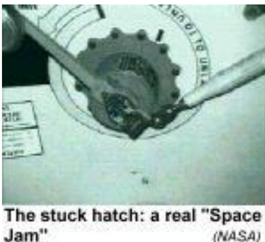
Figure 1.7.3-c Jammed hatch from loose screw
