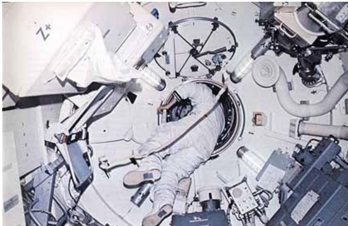
Figure 1.5 Pilot Joe Kerwin shown in the hatch between the Multiple Docking Adapter and the Apollo spacecraft.
